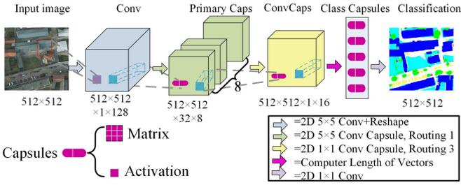
Fig. 4. Simple three-layer Capsule network.
